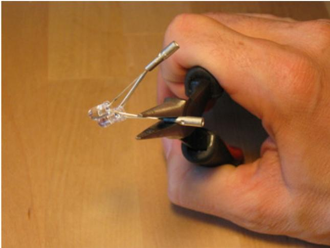
With your pliers, squeeze the splice firmly over the red wire:
