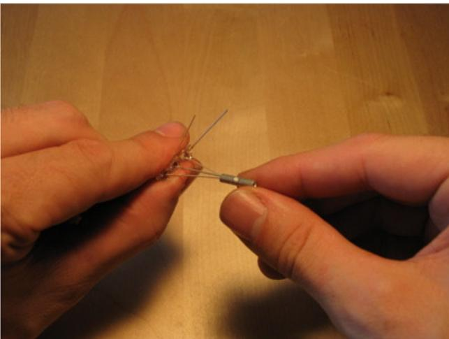
With your pliers, squeeze the butt splice where it encloses the 3 LED leads, being careful not to crimp the opposite side of the splice. Apply enough pressure so that the 3 leads are held solidly in place:
