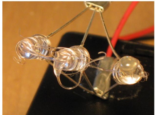
Let the glue cool, and see how it looks when projected against the screen. Give it a few minutes to let the LEDs cycle through their various colors. Feel free to experiment, as it's easy to peel the cooled glue off the lens and try something different!
