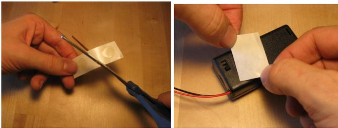
Press firmly, and peel off the backing (if needed, use your finger to help the glue dot stick to the case, but try not to touch the glue more than necessary):
