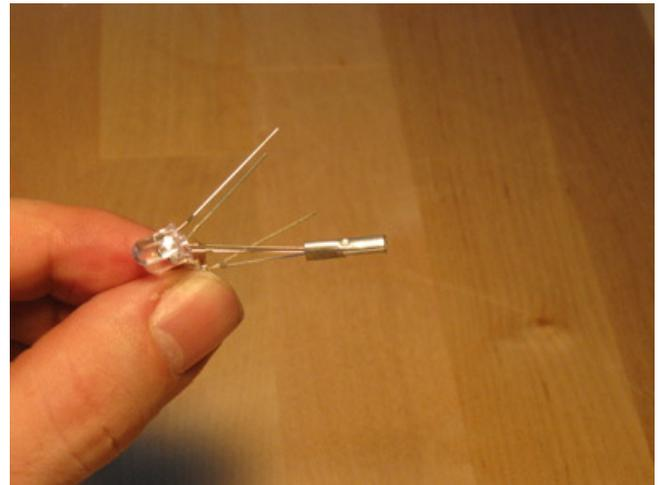
It's very important that you remember which are the positive LED leads; you may want to mark this splice with a small piece of tape. If you get confused, each LED lens has a little flat spot next to the negative lead.
